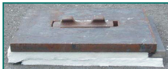
LINER PLATE AND BASE SHOWING FIBRE INSULATION
