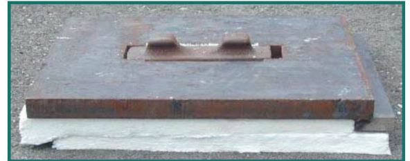
LINER PLATE AND BASE SHOWING FIBRE INSULATION
