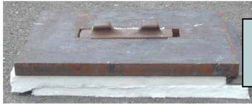
Liner plate and based showing fibre insulation
