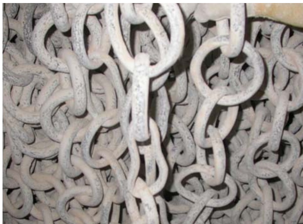
Figure 3. Thinned and warped round-link chain
