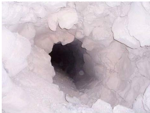
Figure 1. Ring formation in the PRPD lime kiln
